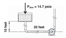
From the Pressure vapor curve with the temperature of 130 °F we determinate the value of the liquid vapor pressure  $P_{vap} = 2.5$  psia = 5.775 feet of  $H_2O$ .
